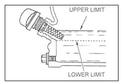
**NOTE:** The pump is fitted with a low oil sensor which will stop the engine if the oil level drops below the safe level to avoid internal damage. Refer to troubleshooting section.
